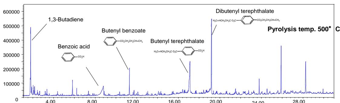
Fig. 1 Pyrogram Obtained by Flash Pyrolysis of PBT
