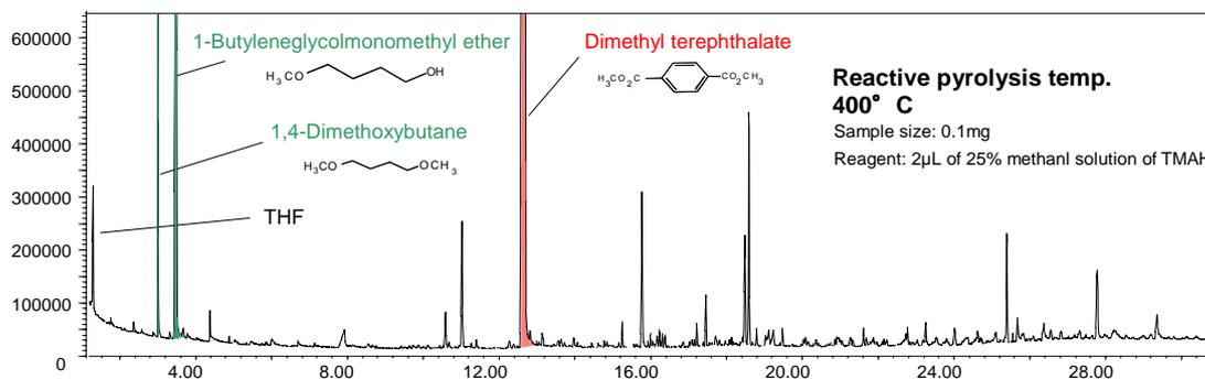
Fig. 2 Pyrogram Obtained by Reactive Pyrolysis of PBT
