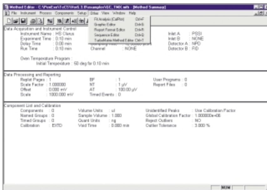
Figure 2. TotalChrom 6.3 Method Editor includes a function to invoke the TurboMatrix RCS Method Editor.
