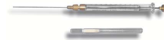
Syringe (top) and liquid-phase calibration tube containing a 1 cm bed of Tenax TA (bottom)
