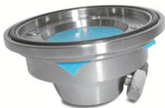
Latex sample secured in the permeation accessory
