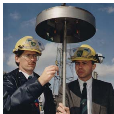
Deploying diffusive samplers for fence-line monitoring.
