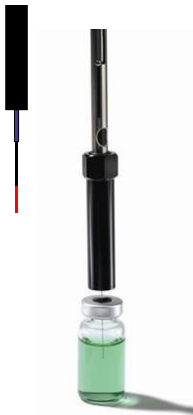
Assembled SPME fiber and holder with fiber immersed in a liquid sample.
