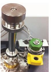
The Agilent 5975T Low Thermal Mass (LTM) with the Thermal Separation Probe (TSP) is the perfect instrument for this task either in the lab or in the field. The TSP requires little or no sample preparation, just measure the sample and start the run. The 5975T LTM GC/MSD utilizing short narrow-bore capillary columns with a quick ramp heating oven rate and fast cooling cycle provides, further improves run times to create an ultra-fast sample cycle.
