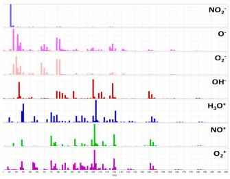
Multi-component gas mixture (subset of the US EPA TO-15 method) analyzed with seven reagent ions
