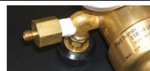
Tank Regulators must terminate in a 1/8" Swagelok® fitting
