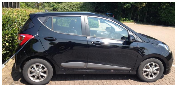
Figure 2 – Vehicle under test conditions. Note the tubing exiting from the rear door on the left of the picture.
