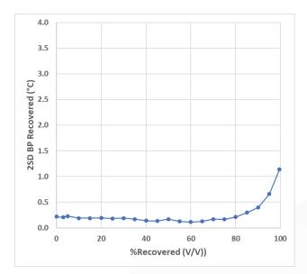
Figure 8. Repeatability (as 2sigma) for DHA to D86 for Naphtha (n=10)
