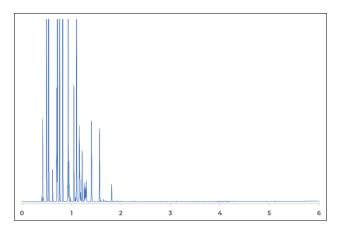
Figure 1. DHA to D86 chromatogram: Naphtha
