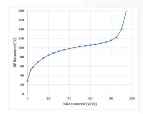
Figure 5. DHA to D86 derived TBP: Alkylate
