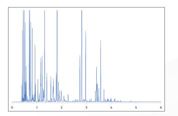
Figure 1. DHA to D86 chromatogram: Gasoline
