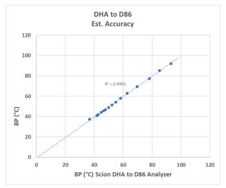
**Figure 7**. Correlation Plot. Obtained TBP vs reference sample data as provided: Naphtha (n=10)
