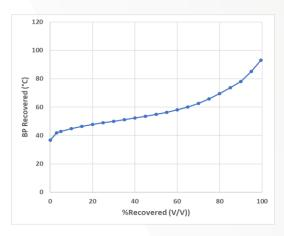
Figure 4. DHA to D86 Derived TBP: Naphtha
