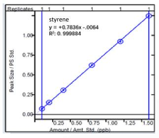
Figure 1d. Calibration curve of styrene
