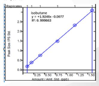
Figure 1a. Calibration curve of isobutane
