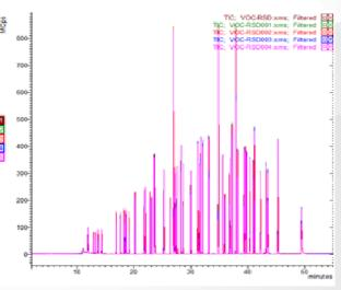
Figure 4. Chromatogram overlay of 52 ozone precursors (n=5)
