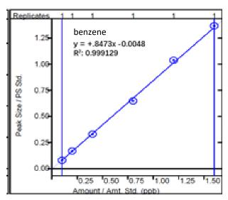
Figure 1c. Calibration curve of benzene
