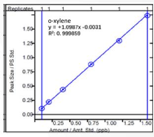
Figure 1e. Calibration curve of o-xylene
