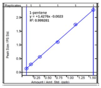
Figure 1b. Calibration curve of 1-pentene
