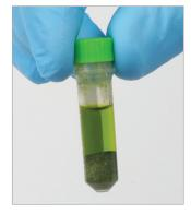
**4.** After centrifugation is complete, transfer the supernatant from the dSPE tube to an autosampler vial, make any final adjustments if required, and test using an appropriate GC or LC method.
