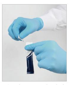
**6.** Open the extraction salt packet by tearing straight across the precut slit.
