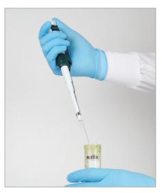
8. Open the cap of the 50 mL tube and add internal standards per reference [1]. Standards are available from Restek.
