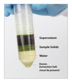
**9.** Confirm that four layers are present to ensure the extraction occurred correctly, and then proceed to instructions for Stage 2: Sample Cleanup [Page 8] or analyze the sample without cleanup.
