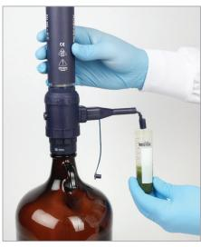
3. Add 15 mL of a 1% acetic acid solution in acetonitrile (v/v).
