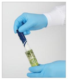
7. Open the cap of the 50 mL tube from step 5 and pour in the entire contents of one packet of extraction salts.
