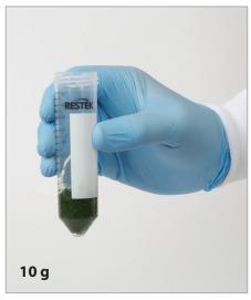
2. Open the cap of a 50 mL centrifuge tube and weigh in 10 g of homogenized sample. Note that the 10 g sample size is for matrices >80% water. For drier materials, consult the method or other resources.
