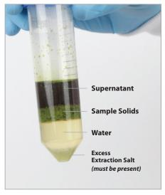
**11.** Confirm that four layers are present to ensure the extraction occurred correctly, and then proceed to instructions for Stage 2: Sample Cleanup [Page 8] or analyze the sample without cleanup.
