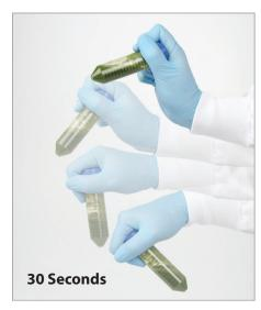
9. Immediately recap the 50 mL tube and vortex or shake it vigorously by hand for 30 seconds.
