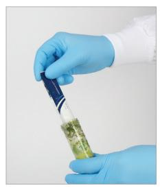
6. Open the cap of the 50 mL tube from step 4 and pour in the entire contents of one packet of extraction salts.
