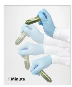
8. Immediately recap the 50 mL tube and vortex or shake it vigorously by hand for 1 minute.
