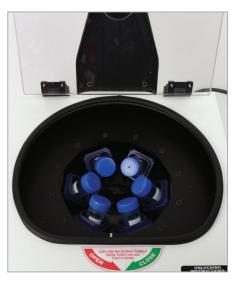
9. Centrifuge the 50 mL tube per reference [2] or [3] to separate the layers.
