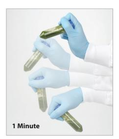
4. Immediately recap the 50 mL tube and vortex or shake it vigorously by hand for 1 minute.
