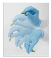
**2.** Immediately recap the dSPE tube and vortex or shake it vigorously by hand (see table for shake time).
