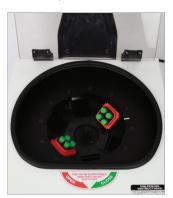
**3.** Centrifuge following the analytical method to separate the solid material.
