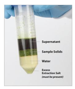
**10.** Confirm that four layers are present to ensure the extraction occurred correctly, and then proceed to instructions for Stage 2: Sample Cleanup [Page 8] or analyze the sample without cleanup.
