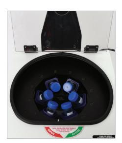
10. Centrifuge the 50 mL tube per reference [1] to separate the layers.
