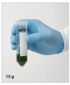
2. Open the cap of a 50 mL centrifuge tube and weigh in 15 g of homogenized sample. Note that the 15 g sample size is for matrices >80% water. For drier materials, consult the method or other resources.
