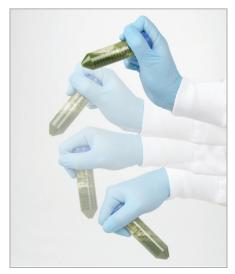
**5.** Immediately recap the 50 mL tube and vortex or shake it vigorously by hand for 1 minute.
