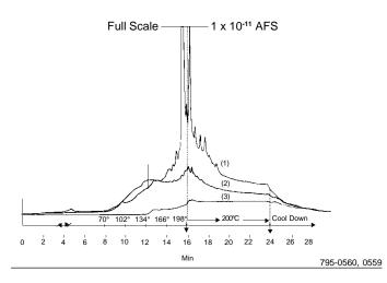
Figure B. Comparative Bleed Curves for High Temperature Septa
