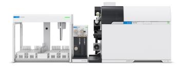
Figure 1. Showing the Agilent 7900 ICP-MS with integrated AVS MS switching valve connected to the Agilent ADS 2 and Agilent SPS 4 autosampler.
