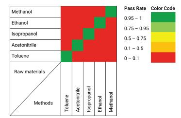
Figure 3. Identification of methanol, ethanol, isopropanol, acetonitrile, and toluene using a SORS challenge matrix.
