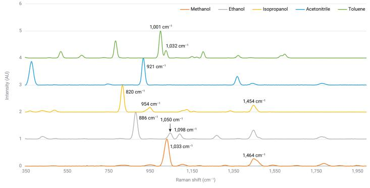
Figure 2. Agilent Vaya Raman SORS spectra of methanol, ethanol, isopropanol, acetonitrile, and toluene. These solvents are often used during the analytical analysis of mAbs or synthesis of oligonucleotides.
