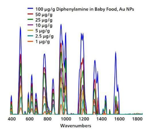
Figure 2. Gold NP SERS spectral profile for diphenylamine in pureed pears, demonstrating detection down to 1 g/g.
