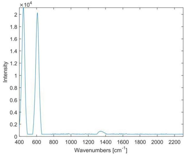
Figure 3. Spectrum of TiO2 (rutile).
