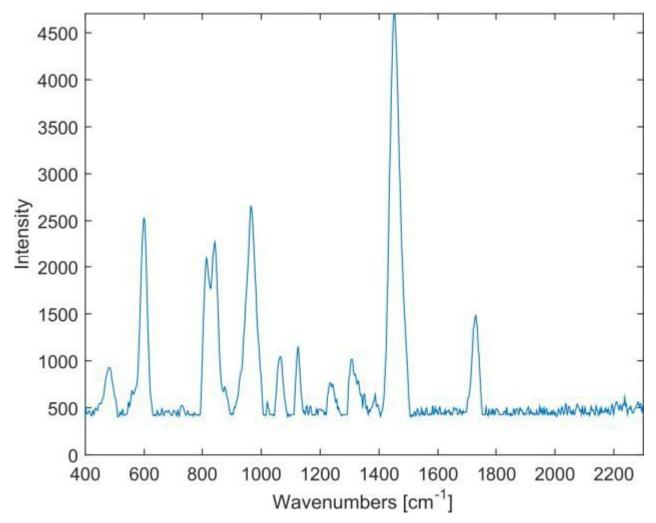
Figure 5. Spectrum of the DEGALAN® resin
