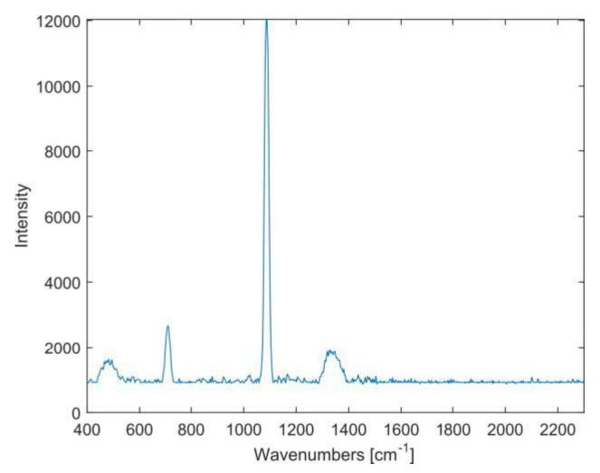
Figure 2. Spectrum of calcium carbonate.
