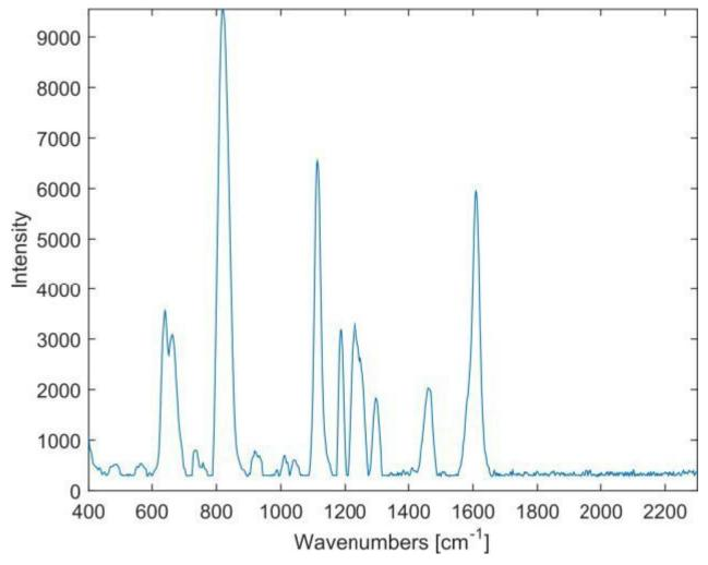
Figure 4. Spectrum of the EPONAC® resin.
