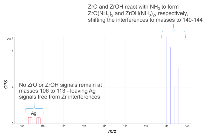
Figure 2. Removal of Zr matrix-based interferences on 107 Ag + and 109 Ag + using the Agilent 8900 ICP-QQQ operating in NH 3 on-mass mode. The interfering ions (ZrO + and ZrOH + ) form reaction product ions which can be seen in the mass spectrum between 140 and 144 u, leaving the analyte ions free of interferences.
