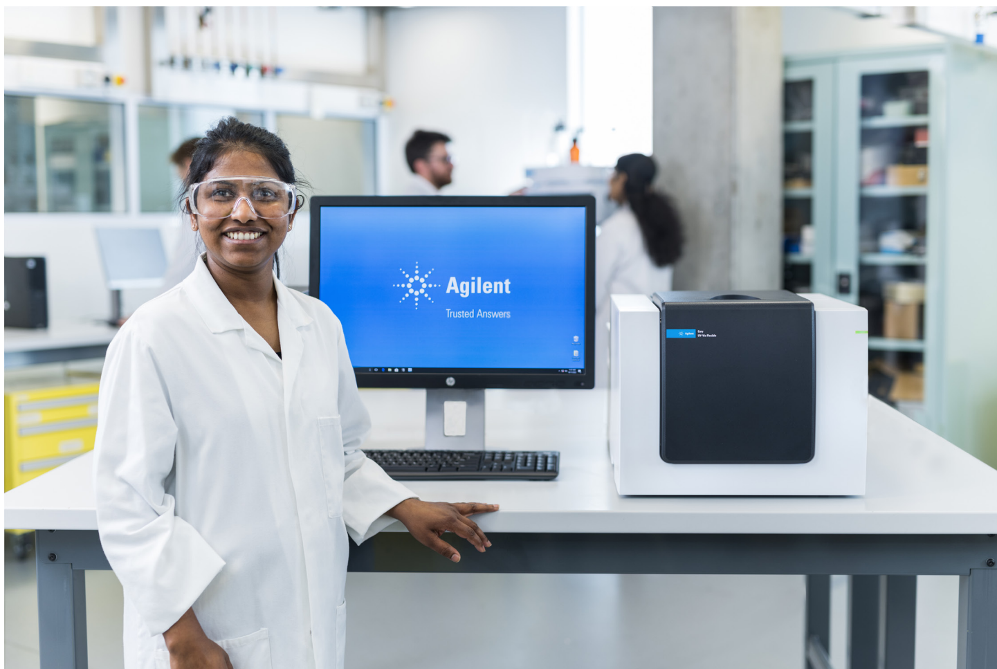
Figure 1. The Agilent Cary 3500 Flexible UV-Vis spectrophotometer includes a large sample compartment and can be fitted with multiple accessories, making it ideal for the characterization of solid samples.
