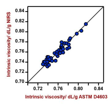
**Figure 3.** Correlation diagram and the respective figures of merit for the prediction of intrinsic viscosity in rPET using a DS2500 Solid Analyzer. The lab value was evaluated according to ASTM D4603.
