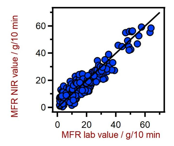
**Figure 3.** Correlation diagram for the prediction of the MFR using a DS2500 Solid Analyzer. The lab values were obtained using a melt flow indexer.
