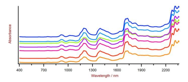
**Figure 2.** Display of a selection of PP Vis-NIR spectra obtained using a DS2500 Analyzer and a rotating DS2500 Large Sample Cup. An offset has been applied to the spectra to make them easier to view.
