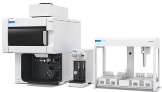
Figure 1. The Agilent ICP-OES Automation System: Agilent 5900 SVDV ICP-OES with integrated AVS 7 switching valve (left), Agilent Advanced Dilution System ADS 2 (middle), and Agilent SPS 4 autosampler (right).
