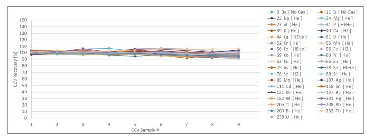
Figure 4. CCV recoveries over the 16-hour analytical sequence.
