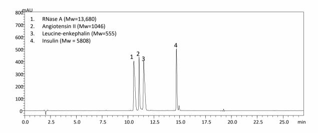
Nexera<sup>™</sup> XR System Column Shim-pack Scepter C4-300 (150 mm  $\times$  4.6 mml.D., 5  $\mu$ m) , P/N:227-31183-05 Mobile phase A 0.1% formic acid in water Mobile phase B 0.1% formic acid in Acetonitrile Flow rate 1.0 mL/min 5 %B(0-2 min) - 5-40%B (17 min) - 95 %B (17.01-22 min) - 5 %B (22.01-27 min) Time program Column temp. Injection volume 5 µL UV 220 nm Detection
