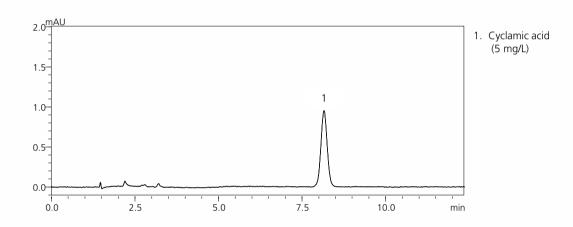
Column : Shim-pack VP-ODS (150 mm L x 4.6 mm I.D., 5 μm)
