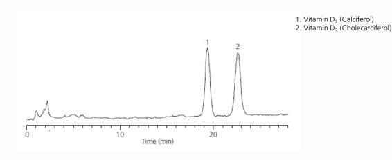
Column : Shim-pack GIS C18-P (250 mm x 4.6 mm I.D., 5 µm), P/N : 227-30557-07
