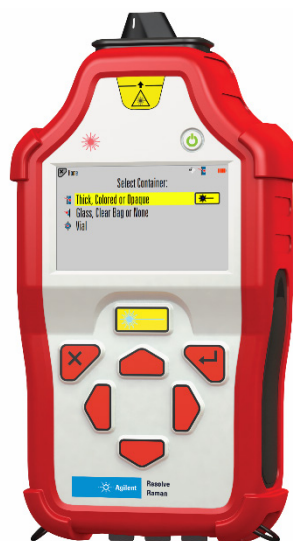
Figure 1. The Agilent Resolve Tactical Analyzer is a versatile through-barrier identification system that can be deployed on location to identify a broad range of materials including drugs, explosives, hazardous toxic materials, etc. Authorities use the portable system to identify a wide range of narcotics and psychoactive substances, as well as other items included in the onboard libraries, in a variety of concealed and obfuscated forms.
