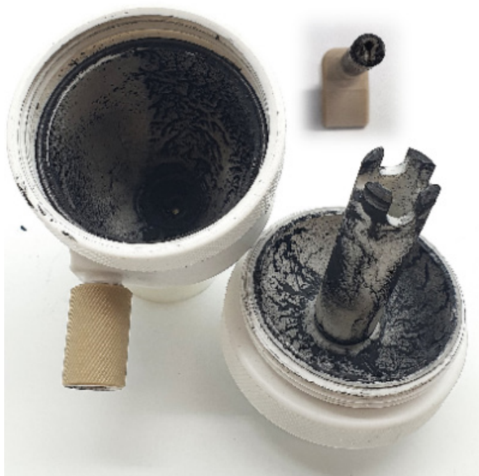
Figure 5. Spray chamber and inert Agilent V-groove nebulizer at the end of the study.
