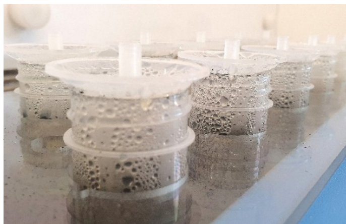
Figure 2. BM samples in the hot block digester.
