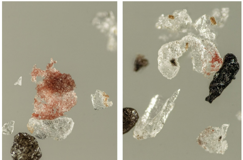
Figure 5. Visual images acquired using the LDIR of PTFE particles after extraction show discoloration, which can reduce visual confirmation during spike-and-recovery checks.
