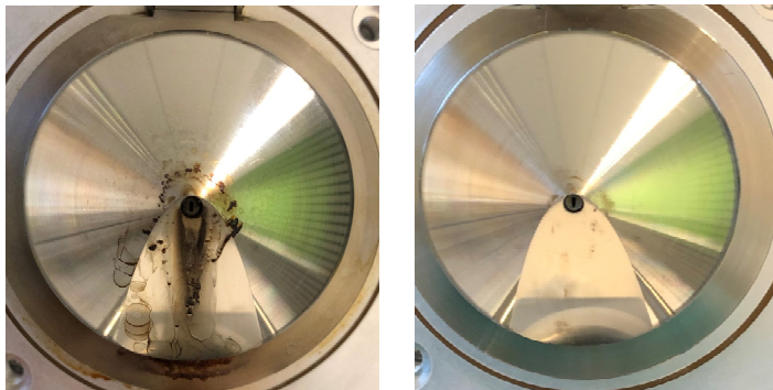
Figure 7. Comparison of inlet cone (~40 test injections): (A) Without matrix elimination, (B) With matrix elimination. Conditions: see Experimental section.
