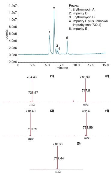
Figure 4. Injection of SST standard 0.28 μg. HPLC method as in Table 1, MS settings as in Table 2. Five peaks are detected in the TIC; the apex peak spectra shows the main component of the peaks. Peak assignment: 1) erythromycin A; 2) Impurity D; 3) erythromycin B; 4) Impurity F plus unknown impurity (m/z 732.4); 5) Impurity E. Impurity D, E, F were tentatively assigned assuming the elution order is the same as in reference 2.
