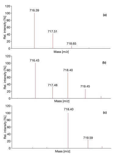
Figure 3. Comparison between spectra of Impurity D (a), impurity D and erythromycin B co-eluting (b), and erythromycin B (c). The quantitation of erythromycin B based on XIC m/z 718.4 is impacted by the isotope of impurity D containing two C13 atoms, in case of coelution.
