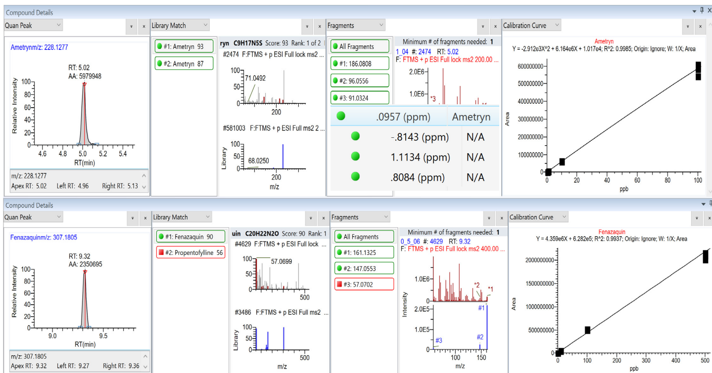
Figure 8. Quantitation ions and confirming ion in MMS in olive oil, along with calibration range from 0.5 to 100 (500) ppb in TraceFinder software for ametryn at 1 ppb and fenazaquin at 0.5 ppb, which shows excellent r^2 , MS 2 fragment ion matching. The technique allows for confident quantitation and screening with confirmation well below the MRL concentration.
