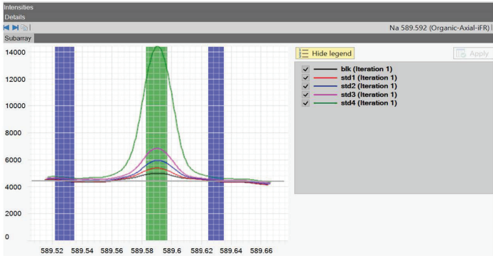
Figure 2. Na standards at 0, 0.02, 0.05, 0.1, and 0.5 mg/L spiked in NMP at an oxygen flow rate of 50 mL/min.
