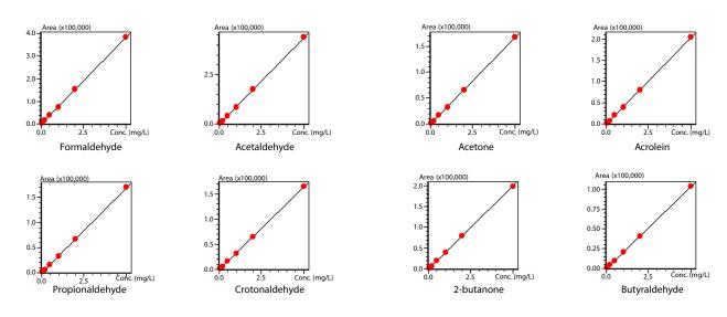
Fig. 3 Calibration Curves for Eight Carbonyl Compounds
