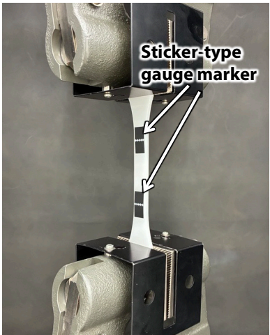
Fig. 3 Enlarged View of Test Setup
