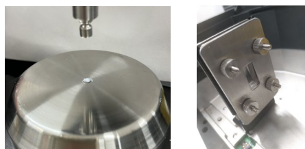
Fig. 2 Left: Sample Applied to Prism, Right: Liquid Cell
