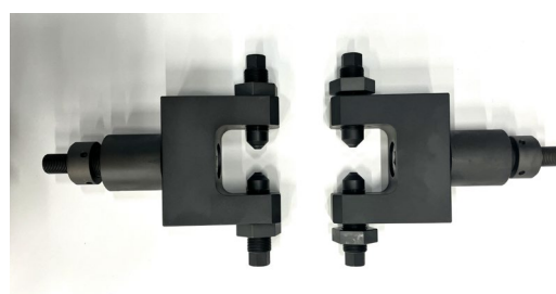
Fig. 3 Shock Absorber Fixtures
