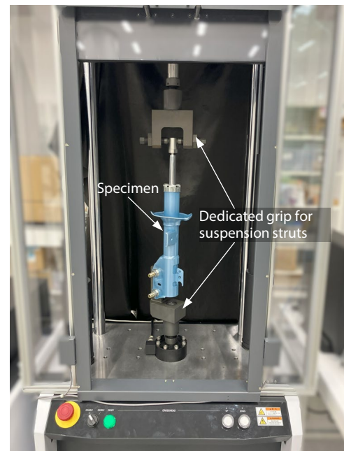
Fig. 2 Specimen Attached to Testing Machine
