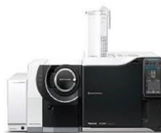
Fig. 1 GCMS-QP™ 2020 NX with EGA/PY-3030D
