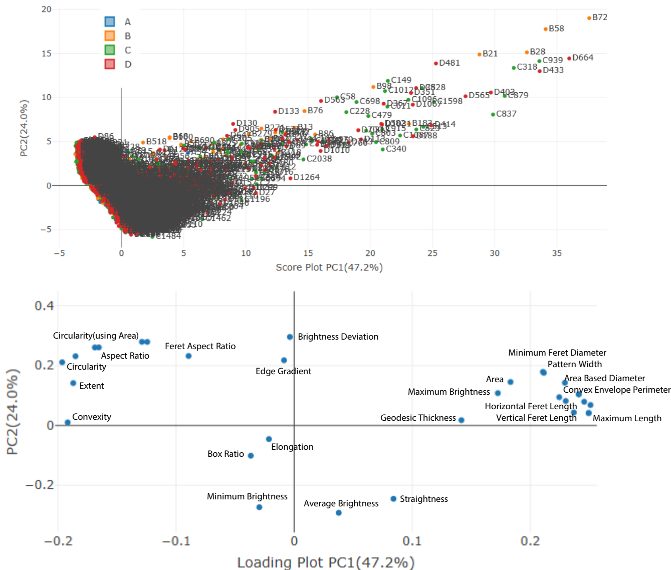
Fig. 9 Visualization of particle shape distribution by principal component analysis
