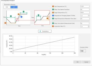
Fig. 5 Temperature Program Setting Window
