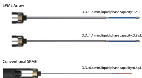
Fig. 1 Comparison of SPME Arrow and Conventional SPME Fiber
