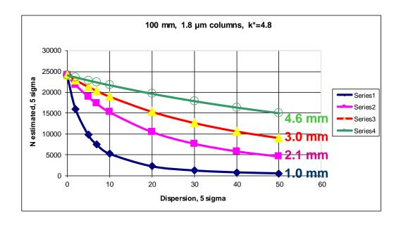
Use the largest columns suitable for the application requirements -- they are less affected by extracolumn contributions. At the same time, consider solvent consumption and detector (ELSD, MS, etc.) compatibility.
