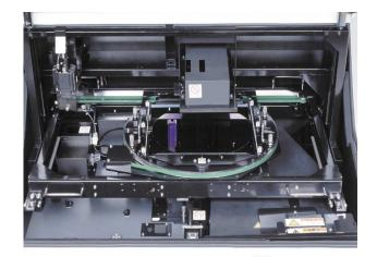
Fig.3 12-inch Wafer Set on Automatic X-Y Stage
