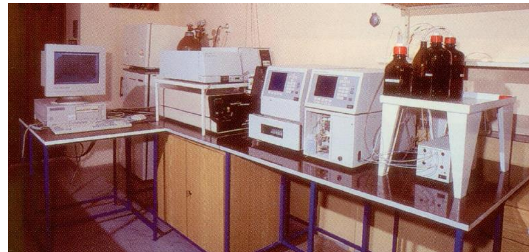
Waters 600 pump, 717 autosampler, 410 RI detector; Wyatt DAWN MALS; SYNPO nineties od last century.
