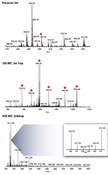
Figure 2. SPS facilitates the isolation of several MS<sup>2</sup> fragments simultaneously, resulting in increased reporter ion signal in the MS<sup>3</sup> spectrum and improving the depth of quantitation significantly.
