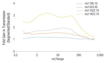
Figure 3. Improved selectivity of precursors with adoption of segmented quadrupole.
