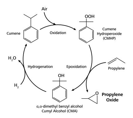
Figure 7. Chemical process behind the cumene route to produce propylene oxide.<sup>5,7</sup>
