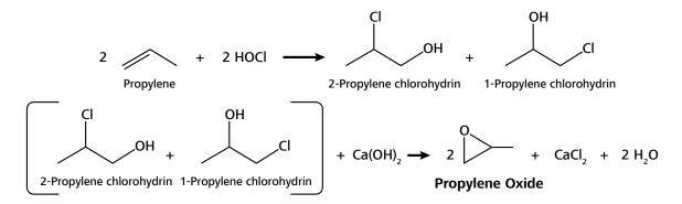
Figure 1. Chemical process behind the chlorohydrin route to produce propylene oxide. Adapted from Bernhard et al.<sup>3</sup>
