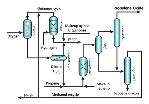
**Figure 11.** Schematic process diagram outlining the hydrogen peroxide-propylene oxide (HP-PO) method for byproduct-free production of PO. Adapted from Nijhuis et al.<sup>2</sup>
