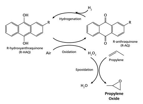
Figure 10. Chemical process behind the hydrogen peroxide route to produce propylene oxide.<sup>5</sup>
