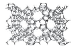
**Figure 9.** Structure of TS-1, Si (grey) and Ti (black) tetrahedral connected via oxygen bridges (white).<sup>8</sup>
