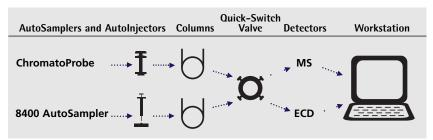
**Easy switching.** In this example, a Varian CP-3800 GC is configured with ChromatoProbe and a standard injector plus a Quick-Switch Valve, a simple, inert column switching valve for column and detector selection.
