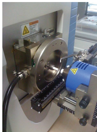
FIGURE 3. DART SVP ionization source attached to a Q Exactive system. The tweezer is showing a lid gasket sample shortly before sampling.
