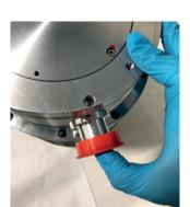
Place the screw back into place (use a 1.5 Nm torque)
