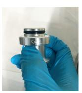
Make sure the o-ring is intact, and then install the provided foreline flange (PN X3511-68001) on the pump
