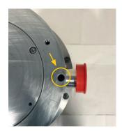
Turn the pump upside down and remove screw from its location
