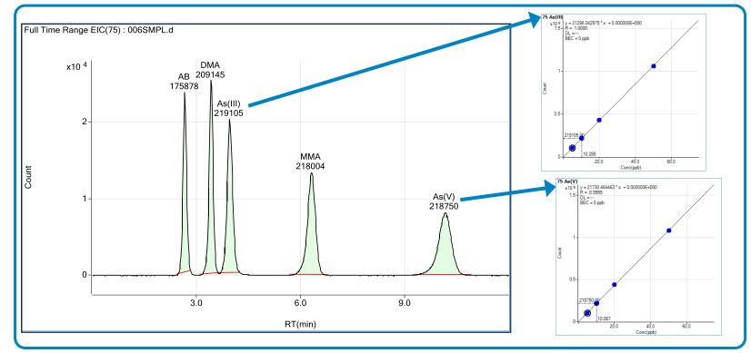
The chromatogram and calibration plots for As(III) and As(V) by LC-ICP-MS with the Agilent 1260 LC and Agilent 7700x ICP-MS illustrate the fast (less than 12 minutes) and complete separation of both As(III) and As(V) from the organic As species.
